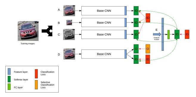
Figure 2: An overview of our proposed model (best viewed in colour). (A) Vehicle identity branch (B) Multi-scale analysis branch (C) Grayscale analysis branch (D) Vehicle orientation branch (E) Consensus learning through feature fusion. Feed-forward signals shown in black. Hard target (groundtruth) loss propagation shown in red. Soft target consensus feedback loss propagation shown in green.
