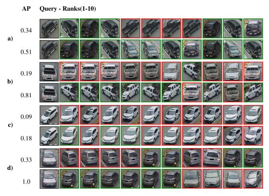
Figure 3: Qualitative comparison of example query images between experiments with and without inclusion of the orientation branch. Rank-1 to Rank-10 is shown. Each pair compares MTML-SG (upper) to MTML-OSG (below) trained and tested on the VeRi-776. AP refers to Average Precision of that query. Correct and incorrect identity matches are shown with green and red borders around images, respectively.
